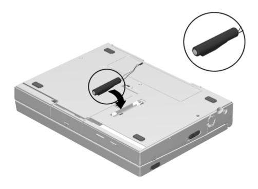
Figure 5-9. Installing the Auxiliary Battery
